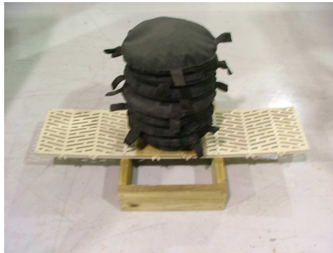
Test #2 Setup – 400 lbs
